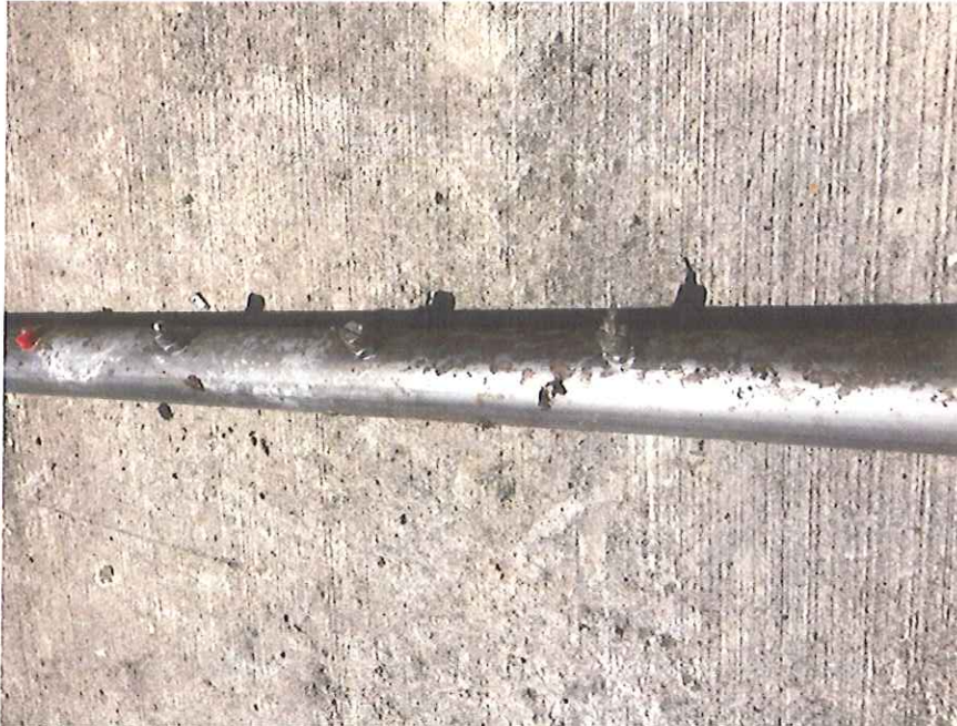
Spray bars with clogged spray heads.
